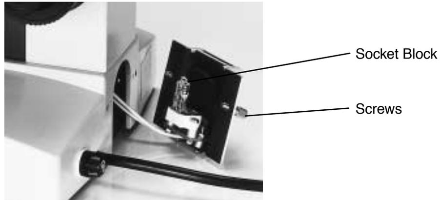
**DO NOT HANDLE WITH BARE FINGERS - BULB MAY EXPLODE WHEN HEATED IF NOT HANDLED CORRECTLY.**
