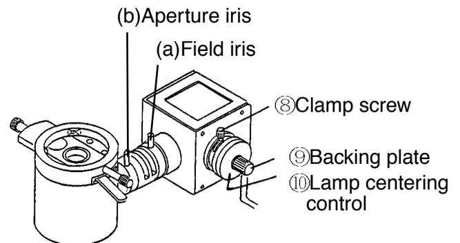
[12] Now adjust the aperture iris (using lever(b) on the Vertical Illuminator), closing it down slowly while observing the field of view. A point will be reached where there is a sudden distinct drop in brightness of the field of view. When this occurs, open up the iris slightly, just until this brightness condition reverses, but no more.
