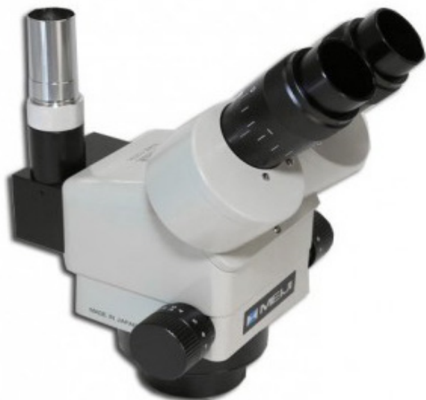
EMZ-13TR (1.0X–7.0X) Trinocular Greenough Design, Stereo Zoom Body, Working Distance 3.5" (90mm)
