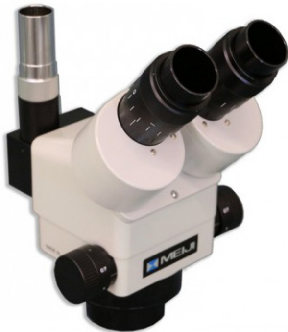
EMZ-8TRU (0.7X–4.5X) Trinocular Zoom Greenough Stereo Body with a Top Light Port, Working Distance 104mm
