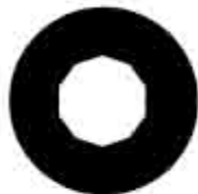
Field of view after Condenser alignment
