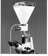
Picture shows Measuring Microscope equipped with PMX100/405, MA582 camera adapter and MA581 vertical illuminator.
