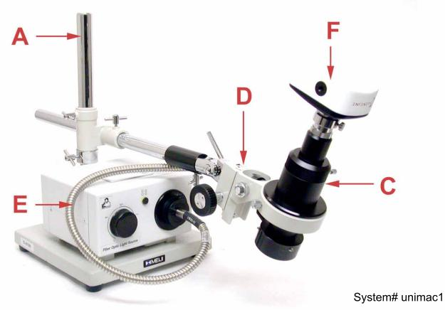
Unlike stereo optics pods which are only using one of the optical paths to connect with a camera, the UNIMAC system is essentially one zoom optics element. And since UNIMAC is modular, there are hundreds of possible configurations, each one tailored to your imaging tasks.
