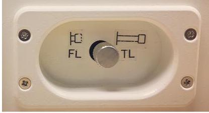
3. On the right side of the MT-B300, make sure the TL Wheel (Brightfield) is scrolled down to its lowest position.
