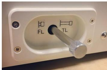
4. On the left side of the MT-B300, make sure the Fluorescence control Wheel (FL) is scrolled down to its lowest position.
