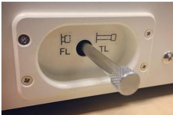
**Note:** Focus objectives by moving focusing wheel in front of the MT-B300. To control light intensity to TL (Brightfield Mode) move the wheel from the right side of the MT-B300 up or down.
