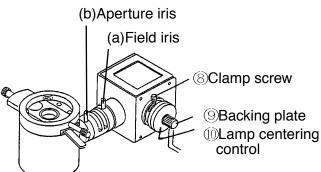
[12] Now adjust the aperture iris (using lever(b) on the Vertical Illuminator), closing it down slowly while observing the field of view. A point will be reached where there is a sudden distinct drop in brightness of the field of view. When this occurs, open up the iris slightly, just until this brightness condition reverses, but no more.
