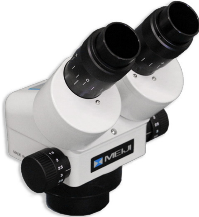
EMZ-5 (0.7X–4.5X) Binocular Greenough Design, Stereo Zoom Body, Working Distance 3.7" (93mm)
