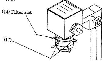
(vii) The models VT·B·2 and VT·T·2 are supplied with the two condensers, one N.A. 0.30, WD 55mm and the other N.A. 0.55, WD 21mm. The N.A. 0.30 condenser is used for 40X objectives. The replacement of the condenser can be done by loosening the three set screws (17)
