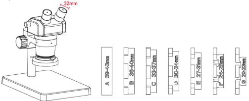
2. For example: eyepiece diameter , choose adapter # D (30-34mm) , put into the chuck, remove the eyepiece, flat on the inner jacket,tighten the swivel.
